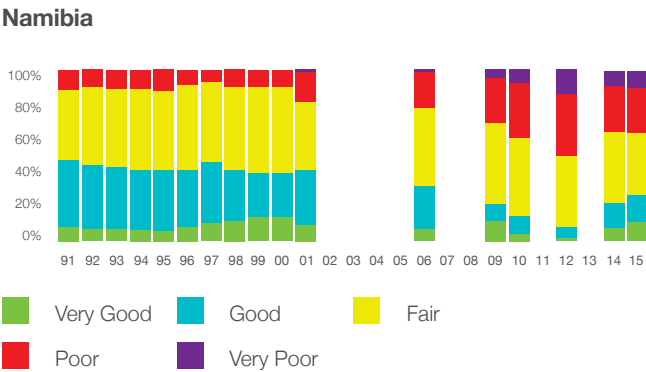
Figure 3 Surfacing Condition (Reseal Need) Change Over Time
